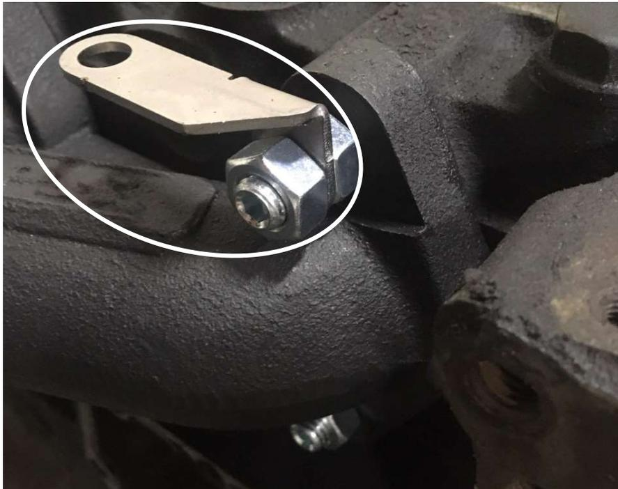
**Step 4:** Now use the **D** bolt and **F** nut to attach the coolant line to the bracket. The coolant line should have a tab that lines up with the **G** bracket
